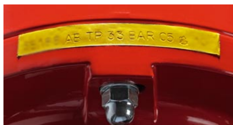
Registration code on the burner's flange
